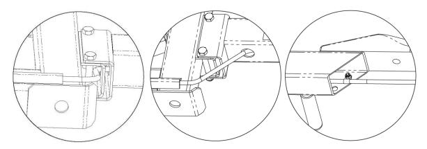
Route the shorter wire cables through the shielded cable runs on the bottom of the frame (under the hydraulic fluid tank). The 36" cable goes to the right hand light, and the 41" cable to the left hand light.
